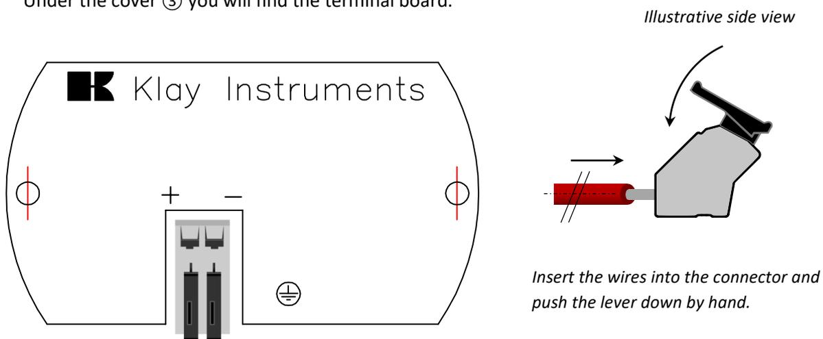
The figure above shows the wiring connection of the transmitter. The 2-wires must be connected to + and - on the terminal board. The wiring terminals can be operated without a screwdriver. The opening levers of the terminals can be lifted and pressed down by hand. Lift the opening levers of the terminals and insert the corresponding wires. Press down the levers by hand, the terminal spring will close and the wire is clamped. *Optionally a secondary 4-20 mA output is available on request.*
